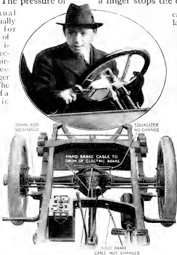
The brake-motor is controlled from the steering-wheel column by simply moving a switch-handle
